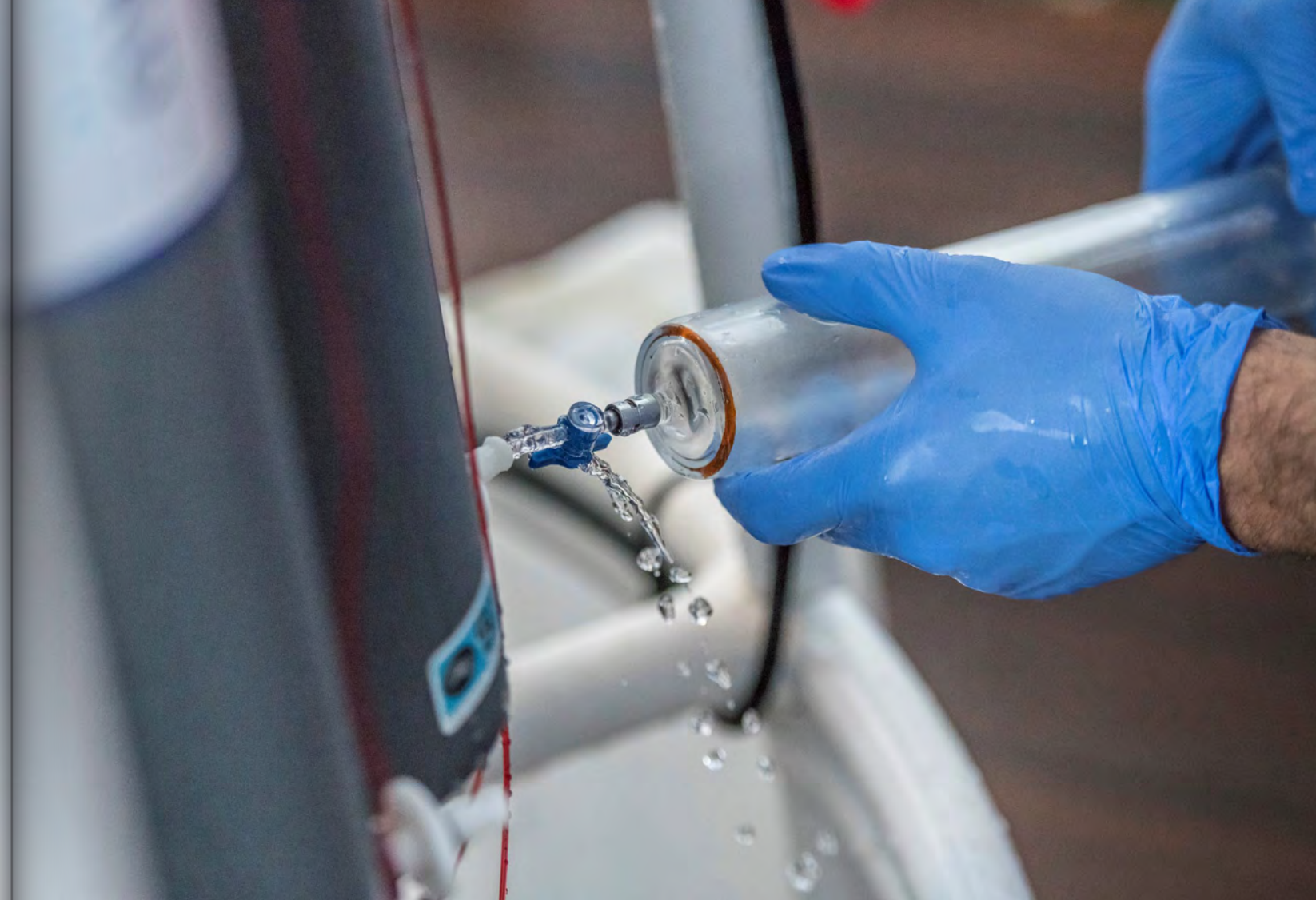
Collecting a CFC-12 water sample from a CTD rosette. Photo by © Christian Clauwers.
